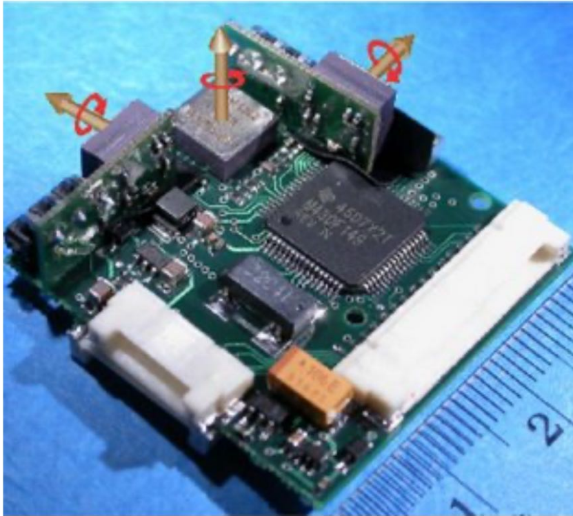
Johns Hopkins Multichannel Vestibular Prosthesis
